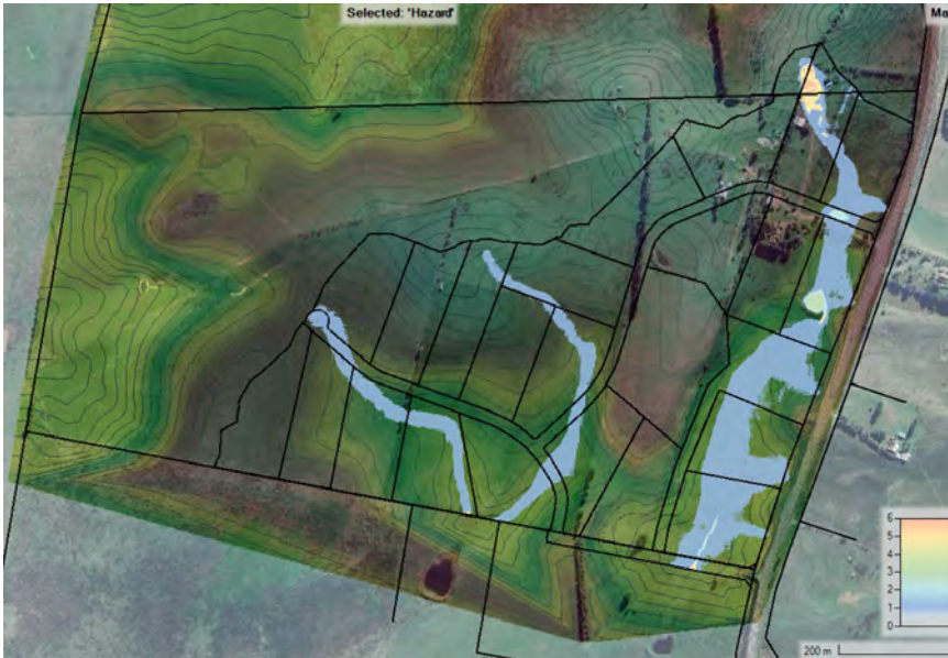
Figure 7: 0.05% AEP Event – ARR2019 Hazard Classification– Pre-Development
