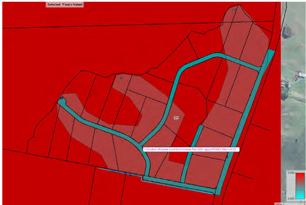
Figure 12: 2D Hydraulic Model – Post Development Manning's Roughness
