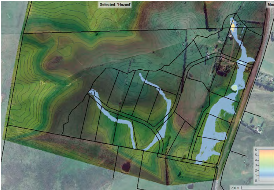
Figure 5: 1% AEP Event – ARR2019 Hazard Classification– Pre-Development
