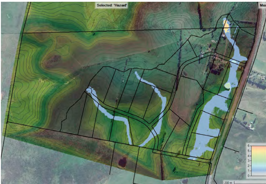
Figure 6: 0.2% AEP Event – ARR2019 Hazard Classification– Pre-Development
